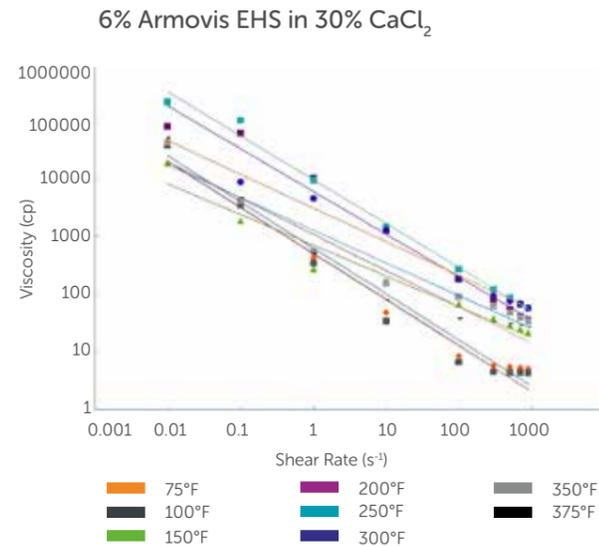
Fig. 5 Example of shear-thinning viscosity of VES fluids
