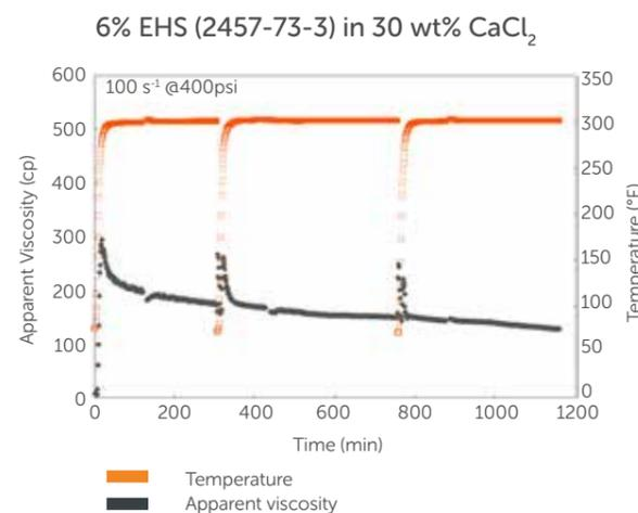
Fig.2 Thermal Stability of Armovis EHS in depleted acid (20% HCl -> 30% CaCl<sub>2</sub> brine) at 300°F
