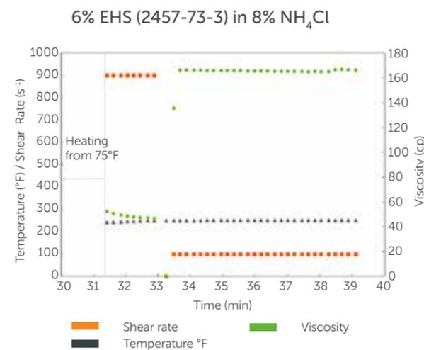
Fig.6 Example of viscoelastic properties of VES fluids (6% VES in NH<sub>4</sub>Cl brine)
