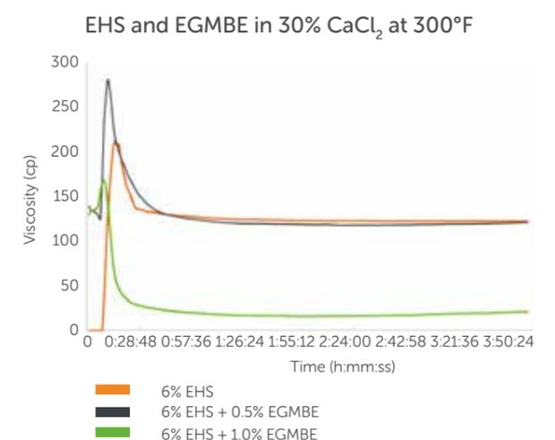
Fig.4 Breaking effect of VES GEL through EGMBE as a mutual solvent post-flush
