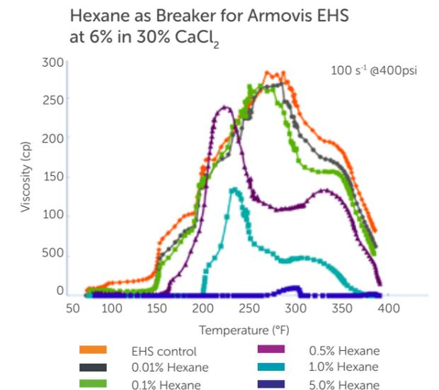
Fig. 3 Breaking effect of VES Gel through the use of Hexane
